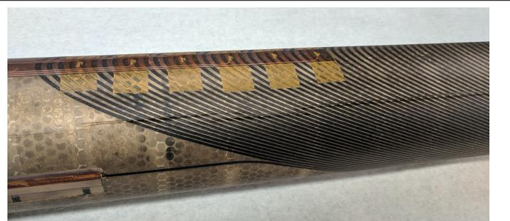
*Figure 3. A single layer of a Nb<sub>3</sub>Sn CCT magnet: each turn of the Rutherford cable is supported by a machined groove in the mandrel. A “trace”, effectively a lithography patterned flexible sheet of Cu-coated Kapton, is seen on top, providing access to voltage taps on the turns of the magnet.*
