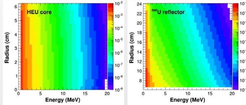
MCNP 6.2 simulations for the neutron flux of Oy Flattop.
