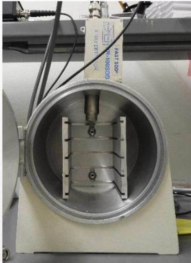
We use high-resolution silicon drift detectors to measure the X-rays from the iridium samples. We determine  $^{193\text{m}}\text{Ir}/^{192}\text{Ir}$  ratio by fitting the three peaks with Voigt functions and correcting the peak areas for the  $^{192}\text{Ir}$  and  $^{193\text{m}}\text{Ir}$  decay.
