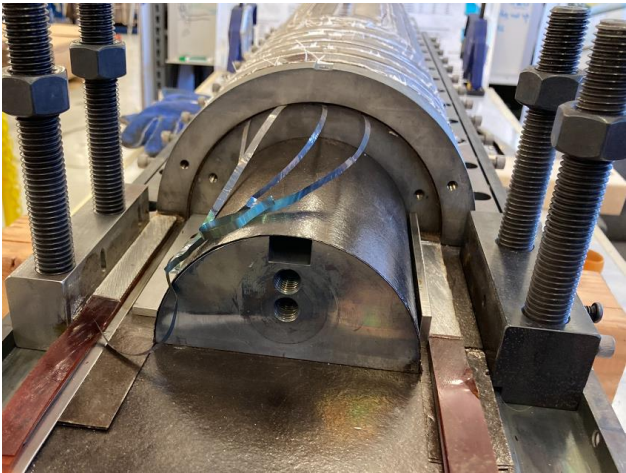
Nb3Sn cable pre-tinning
