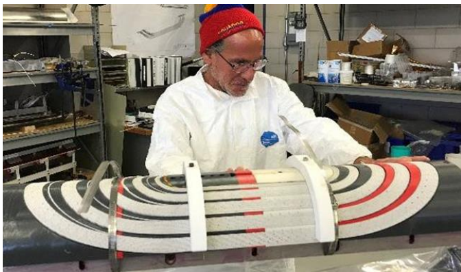
Coil winding process
