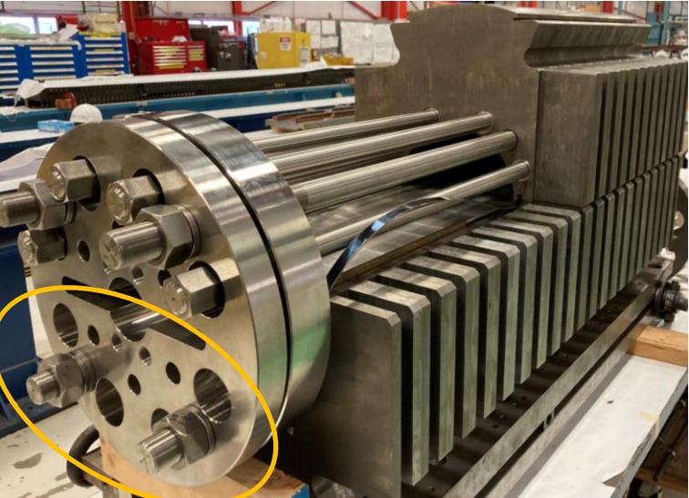
Inner coil support attaching to the iron ends
