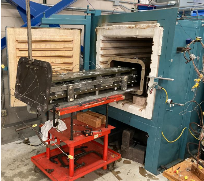
Reaction tooling on the loading cart
