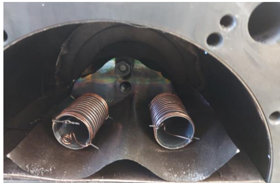
Two witness samples at LE and RE in the reaction fixture
