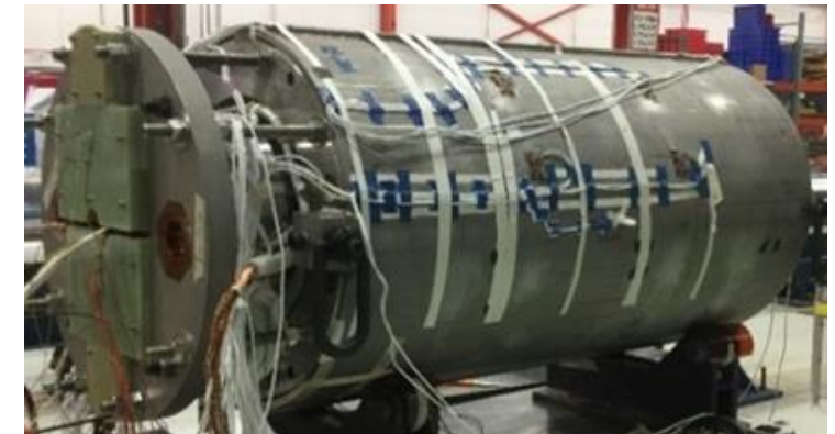
Ends loading and electrical connections*
