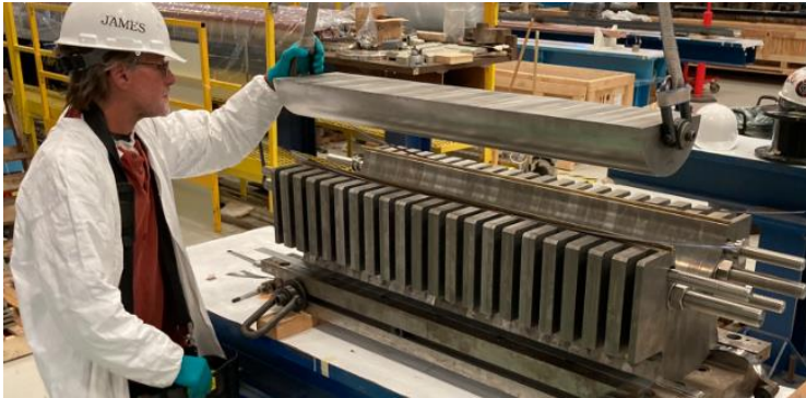
Mirror insertion into the lower yoke
