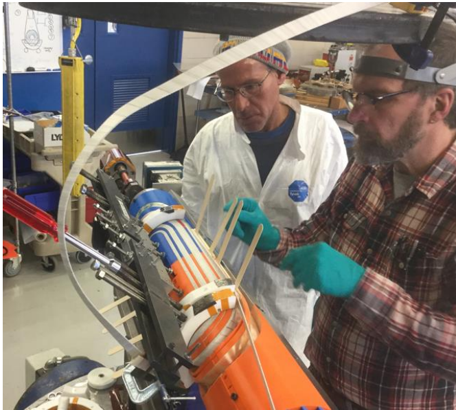
Coil winding process
