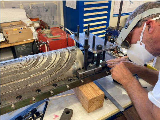
Nb3Sn cable trimming
