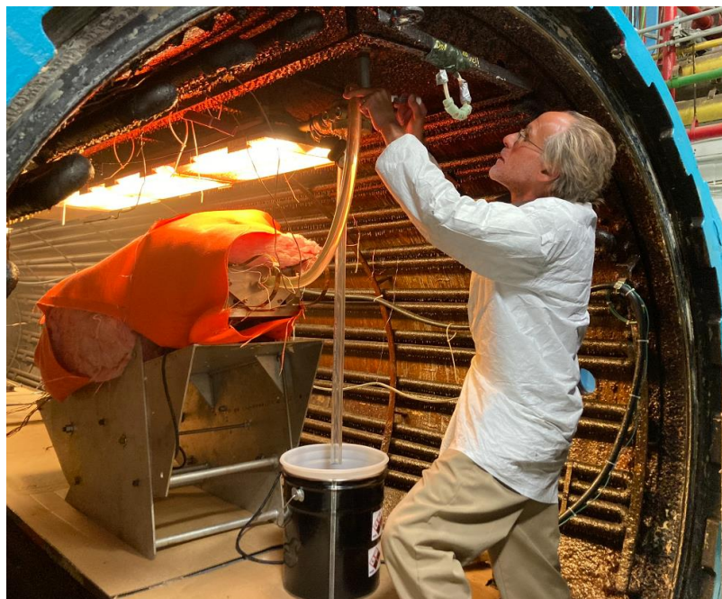
Impregnation setup in the vacuum oven
