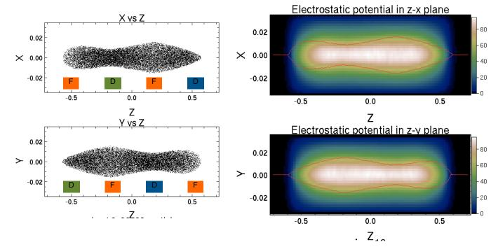
File FODO3D.py - basic 3D simulation of an ion beam in a periodic FODO lattice:
