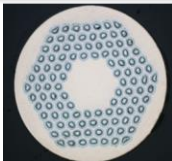
0.7 mm RRP108/127 40-strand cable with SS core
