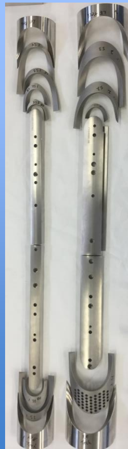
Ti poles and spacers, SS saddles
