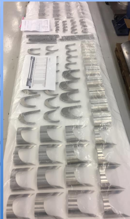
Ti poles and spacers, SS saddles
