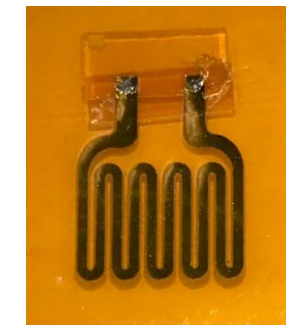
SS spot heater on polyimide substrate; \sim 3 \Omega resistance RT
