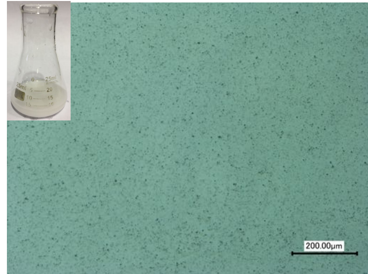
PBA-BNNS disperse well in IPA After 3 h ultrasonic mixing
