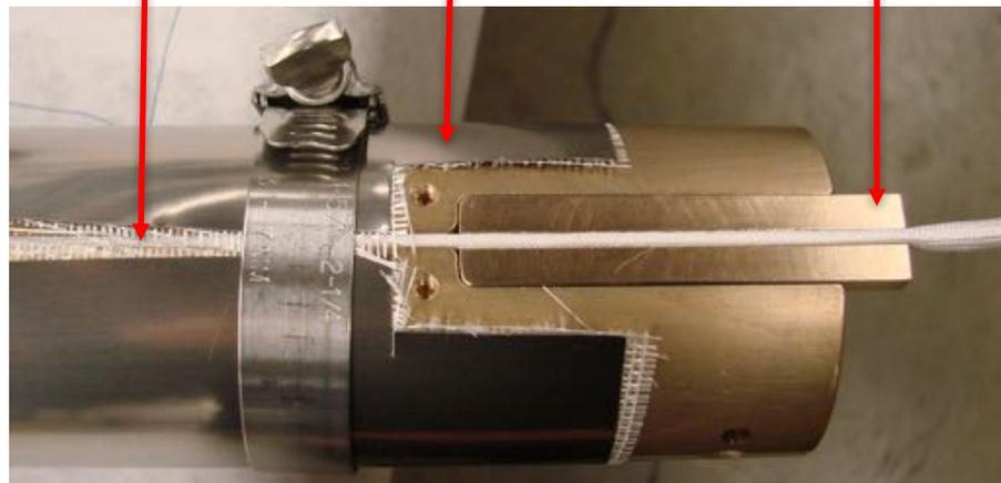
Titanium foil displaced during assembly
