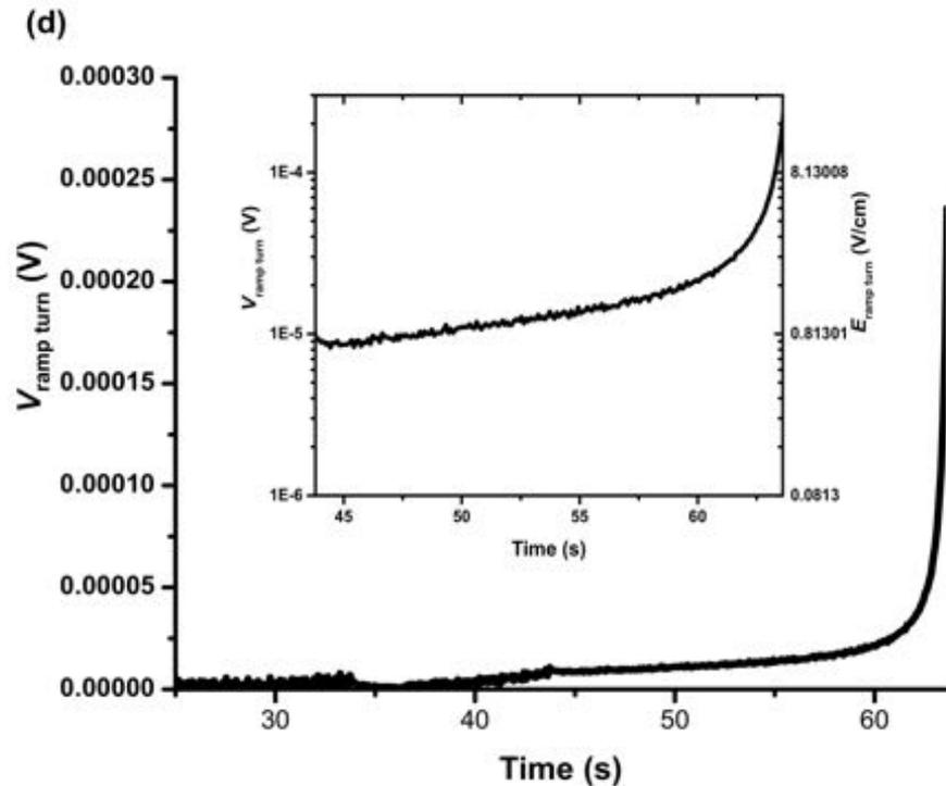
**Ball park analysis – 1.125 J into the ramp turn within  $\sim 15$  s, with the conductor temperature around 14 K.**
