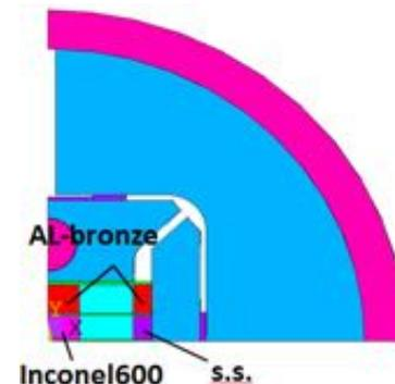
Interference between hor. key and yoke is set to 0.2 mm
