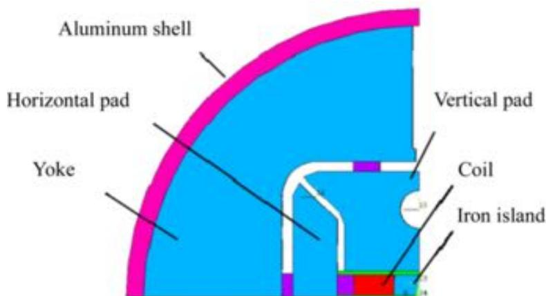
SD01 structure could be modified to fit Nb<sub>3</sub>Sn and Bi-2212 coils for a hybrid magnet producing 15 T peak field at SSL
