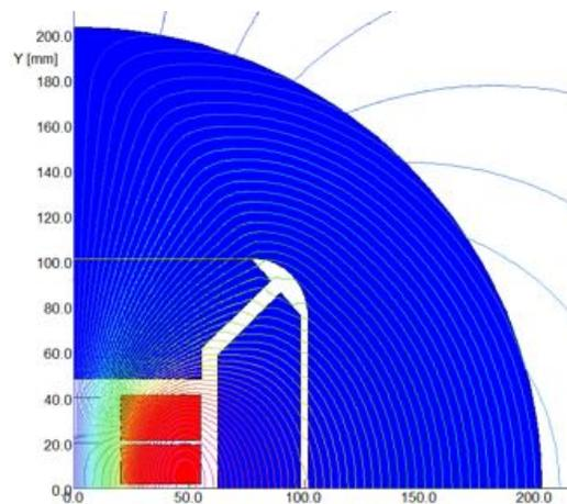
$B_{mod}$  (T) on coils and iron
