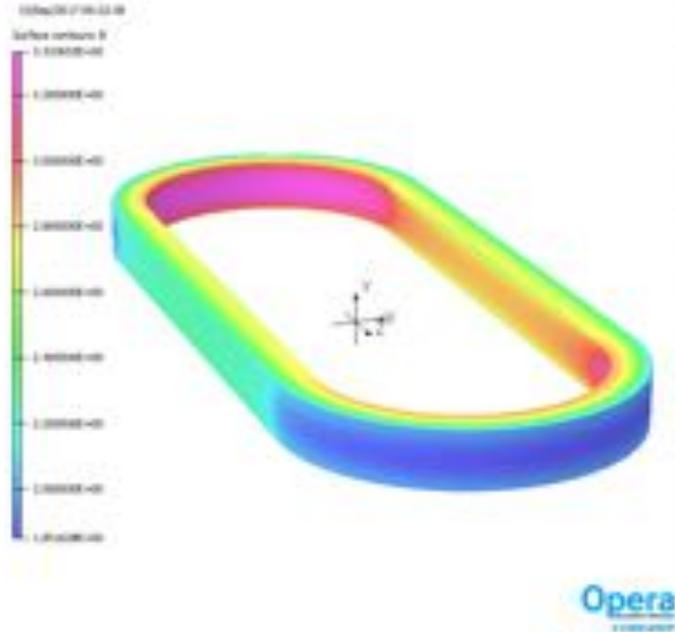
2-layer x 6-turn racetrack coil based on 17-strand Rutherford cable (1.44 mm x 7.8 mm, strand diameter = 0.8 mm)
