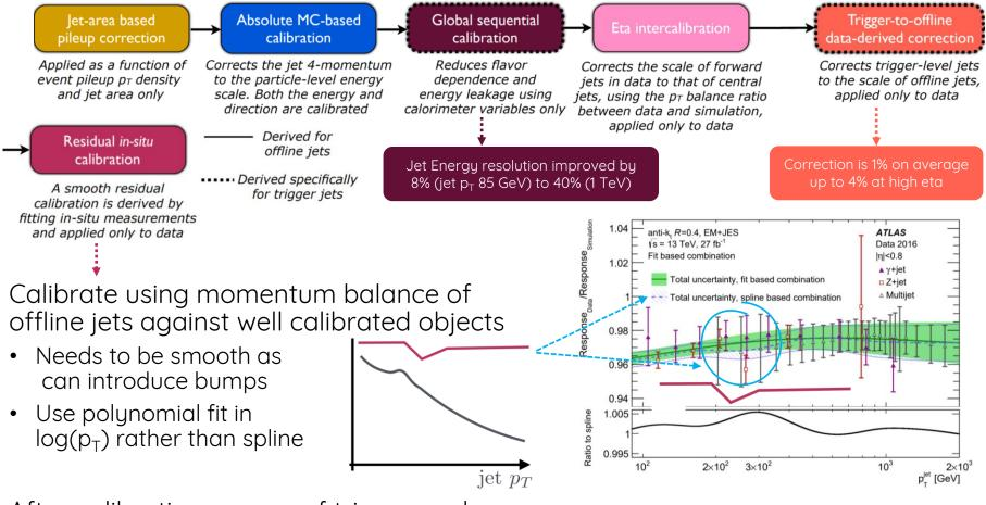
After calibration energy of trigger and offline jets agree within 0.05%
