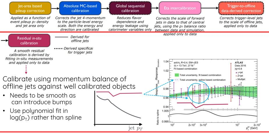
After calibration energy of trigger and offline jets agree within 0.05%
