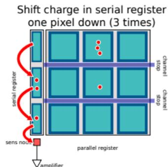
capacitance of the system is set by the SN:  $C=0.05\text{pF} \rightarrow 3\mu\text{V}/e$
