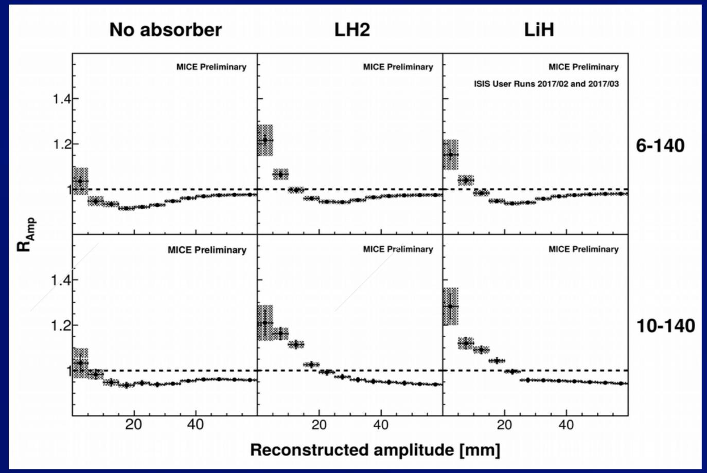
The ratio of the downstream to upstream cumulative amplitudes for two input beam configurations with nominal momenta of 140 MeV/c and nominal emittance of 6 (top) and 10 (bottom) mm. Cooling is observed where R<sub>Amp</sub> > 1, showing migration of muons from high to low amplitude.
