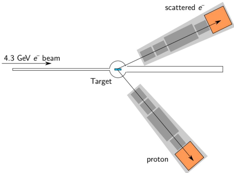
Proton momentum can be determined from coincident detection.
