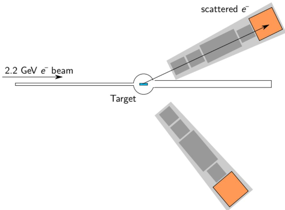
The  $x_B < 3$  experiment used two spectrometers to maximize inclusive acceptance.
