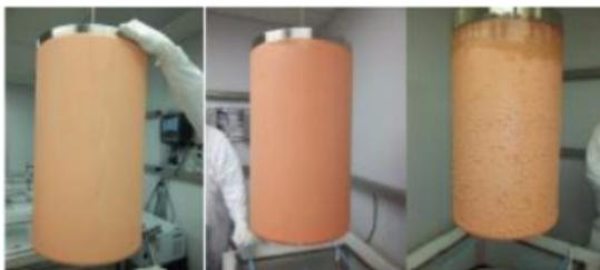
EF copper after turning on lathe
