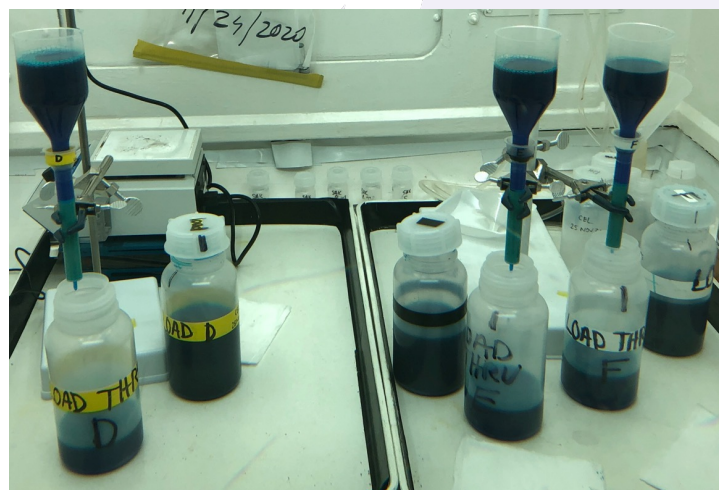
Co removal – 6 column in parallel in 2 hot cells
