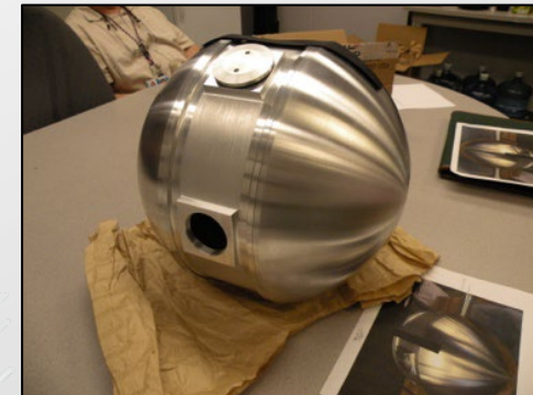
Target chamber for installation in the Gammasphere array
