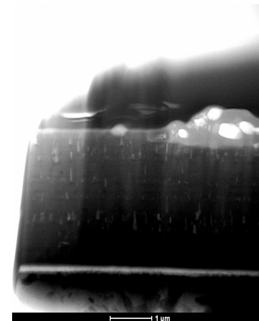
HRTEM of REBCO revealed novel swelling morphology
