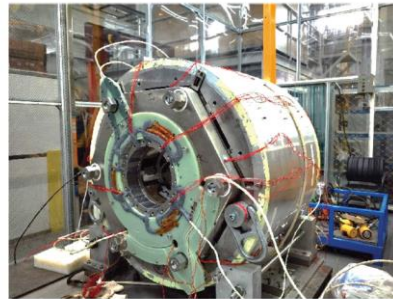
Figure 5: Picture of completed FECR 1/2 size prototype cold mass ready for test.
