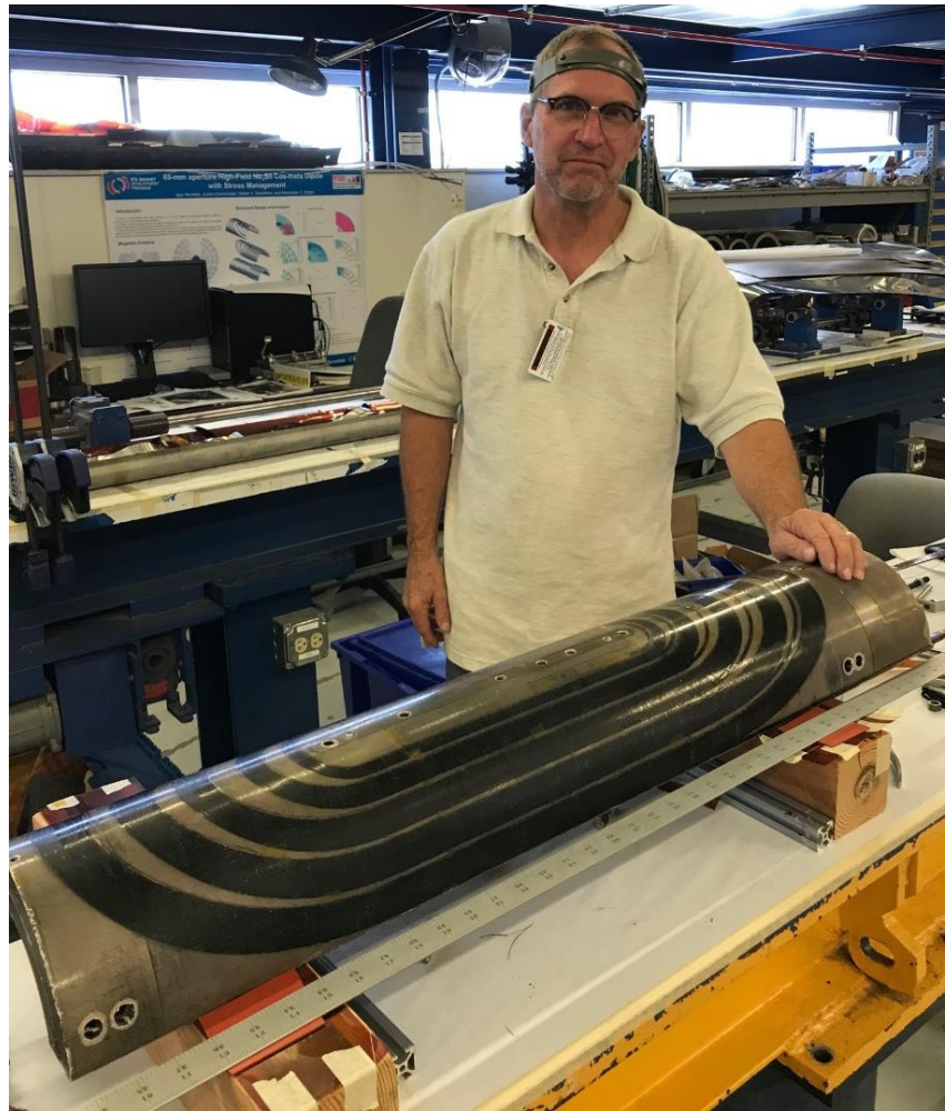
Coil impregnation with epoxy
