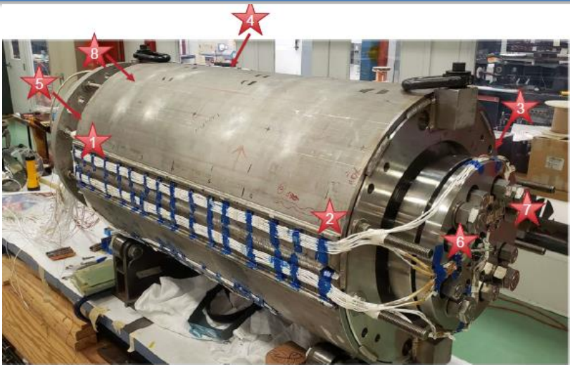
Acoustic sensors location on shell (1-4) and rods (5-8)
