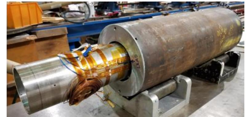
Double-layer tension wrapped and cured
