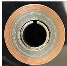
Location of the cutout / superconducting shield tube
