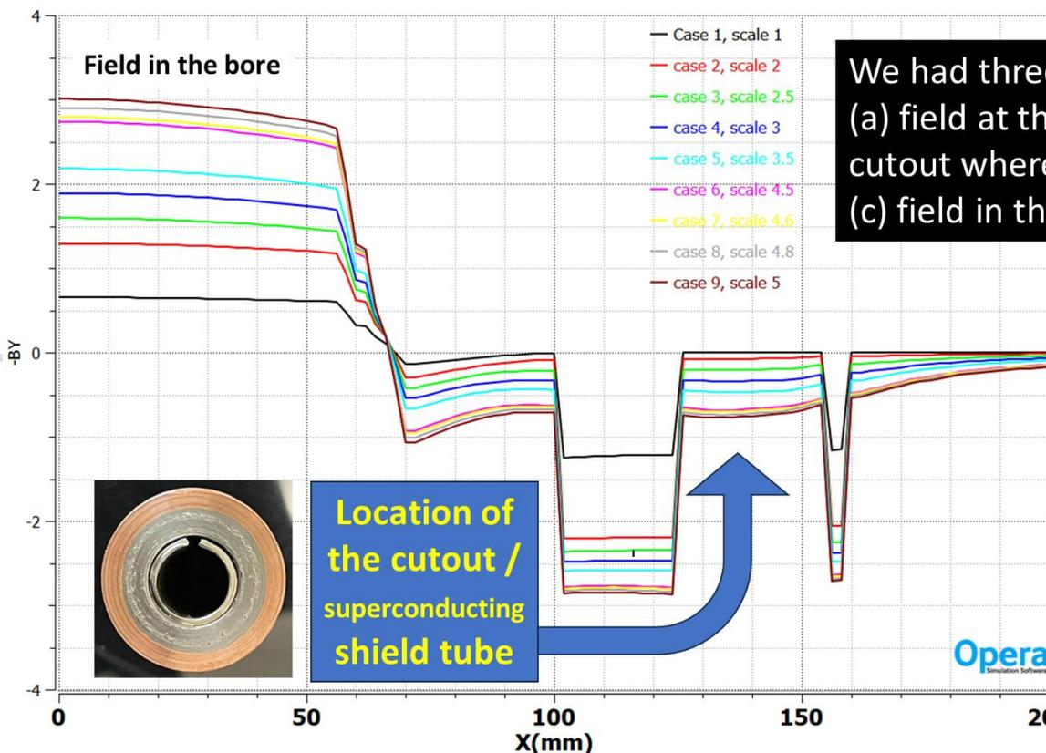
We had three Hall probes to measure (a) field at the center, (b) field in the cutout where the SC shield is (+x) and (c) field in the cutout with no shield (-x).
