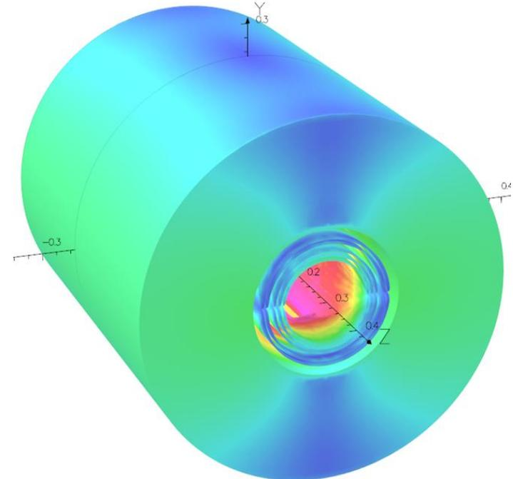
The design is optimized for low field harmonics with the **IntegralOpt** code which also creates OPERA3d input file
