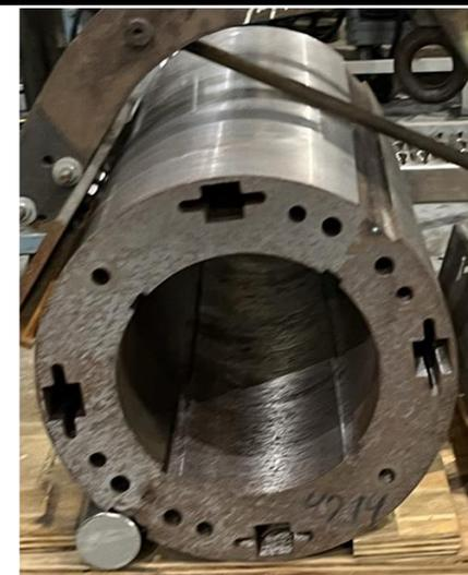
**Field from the high field magnets for ion beams must be shielded on the path of e-beam**
