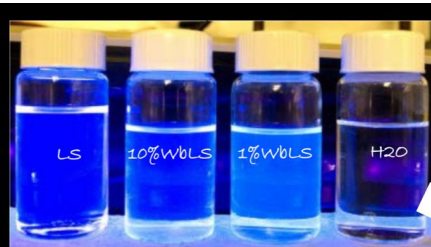
Novel target medium: Water-based Liquid Scintillator
