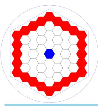
Original plan: 61-Re design: 24 high- $C_p$  + 36 Nb<sub>3</sub>Sn + 1 Cu.
