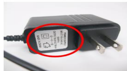
Unlisted power supply
