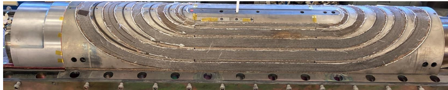
SMCT coil after reaction
