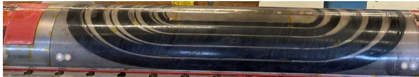
Coil view after epoxy impregnation
