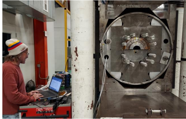
Welding contact tooling for a root pass and weld prep filling
