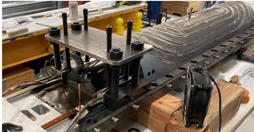
Coil leads splicing
