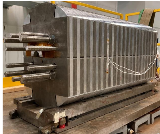
Clamped Iron yoke
