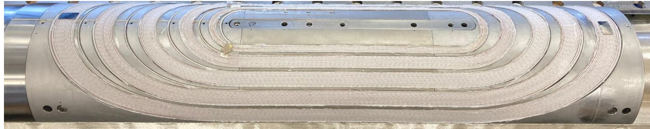
Completed outer layer winding
