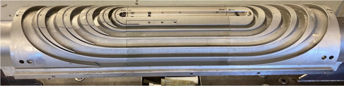
Coil outer layer mandrel before winding
