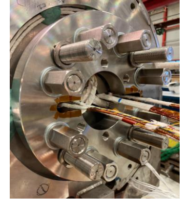
LE end plate for the SMCT coil
