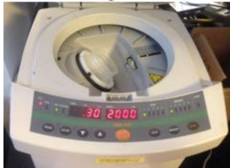
Centrifugal mixer for degassing and mixing fillers into epoxy (@Anderssen lab)
