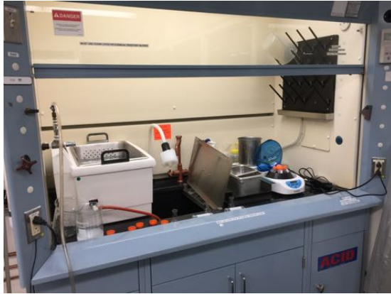
Fume hood for working with nano-matters (w/ ultrasonic bath mixer, centrifuge, magnetic stirrer and hot plate)
