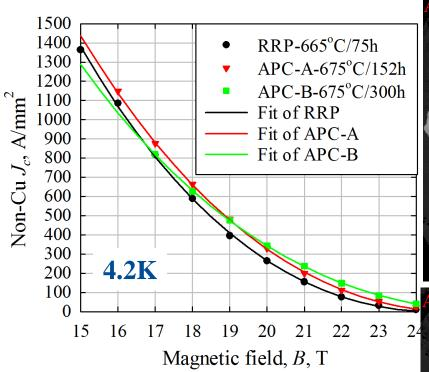
The fitted  $B_{irr}$ s: RRP=24.6 T, APC-A=25.2 T, APC-B=26.2 T, similar to fields at 1% of *R-B*. All wires are above HL-LHC specification. APC-B had low non-Cu  $J_c$  due to low finegrain (FG) Nb<sub>3</sub>Sn fraction.
