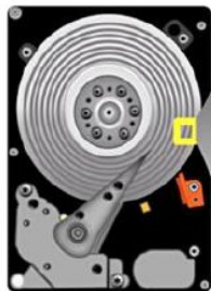
Conventional HDD Data in discrete tracks
