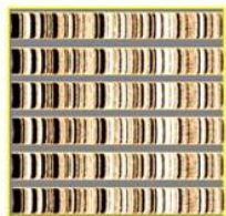
Conventional HDD Data in discrete tracks
