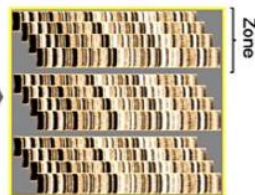
SMR HDD Data in zones of overlapped tracks
