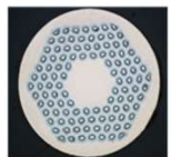
0.7 mm RRP108/127 40-strand cable with SS core
