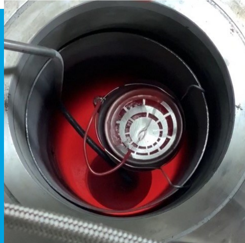
Liquid Fluoride Salt Coolant Flibe ( 2\text{LiF}\cdot\text{BeF}_2 )
