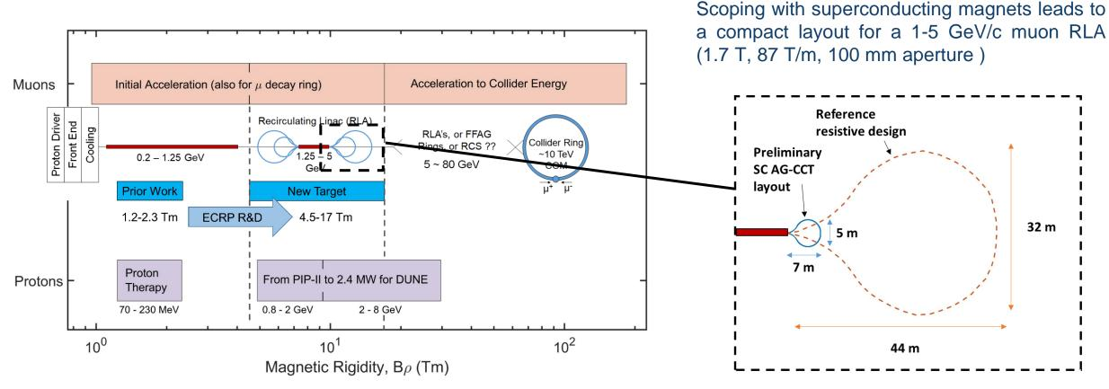
SC magnets reduce footprint with higher field and a novel configuration achieving large momentum acceptance with minimal reverse bending
