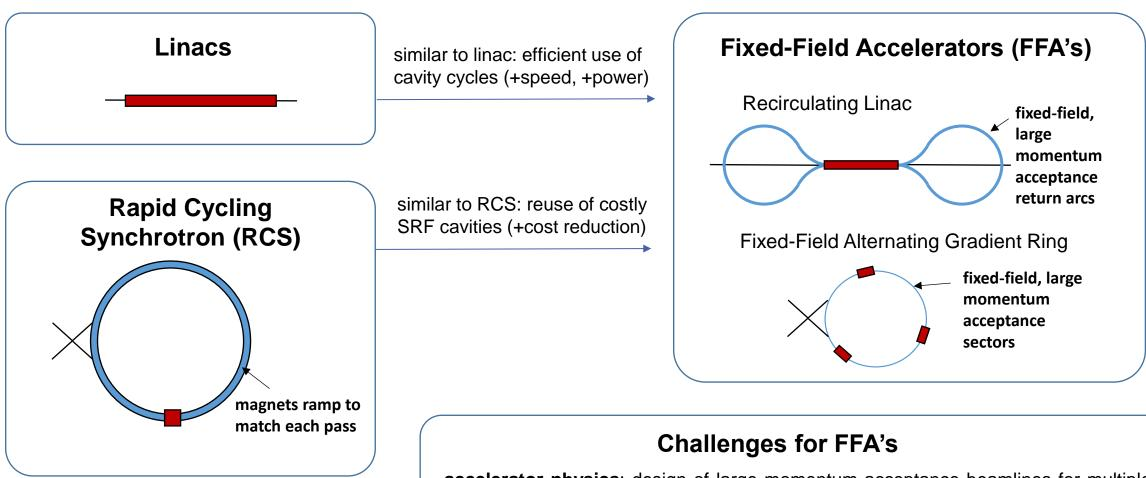
**accelerator physics**: design of large momentum acceptance beamlines for multiple passes with fixed field, tune shift, successful demonstrations so far are for low-energy electrons (e.g. EMMA, CBETA)
