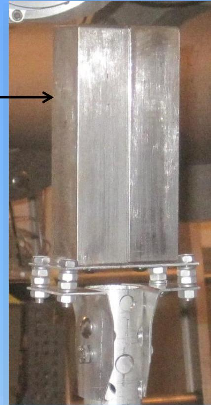
The neutron beam diameter is smaller than the sample size.
