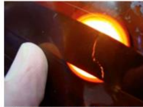
Non detected failure of a QH. As seen after dismounting during inspection of the QH.
