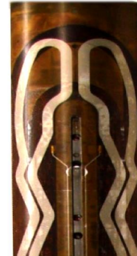
PH strip on top of the HQ-series coil
