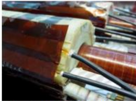
Non detected failure of a QH. As seen after dismounting during inspection of the QH.
