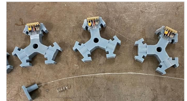
Various AE sensors and mounting hardware (LBNL)
