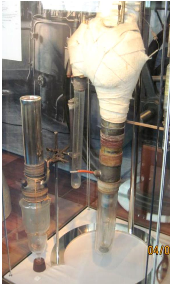
Helium liquefier built in Leiden in 1908 produced ~0.28 liters/hour
