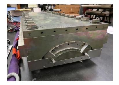
A 0.002" gap between Reaction liner and OD block.
