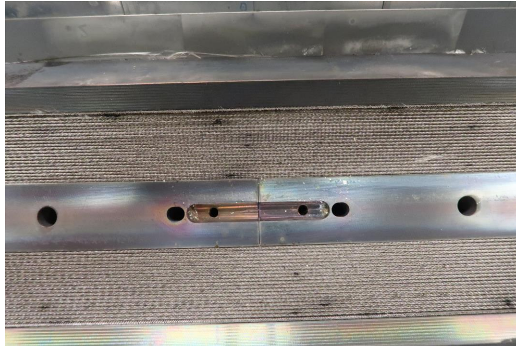
Axial gap between two half poles reduced to 200 micron.
