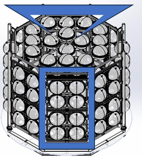
Simply zip tied to the inside of the PSUP frames, with radial liners overlapped
