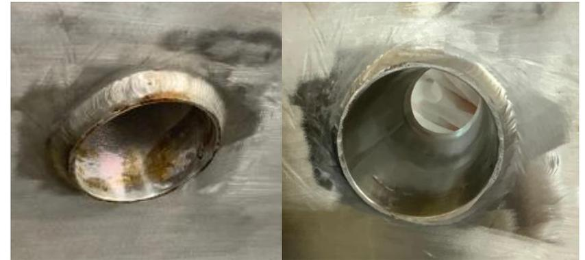
The tank was then inspected, cleaned and passivated in areas with defects. Before the experiment starts the tank will be flushed 3 times
