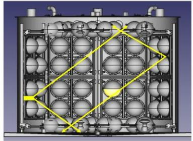
Four diffusers should illuminate each PMT, albeit at different angles
