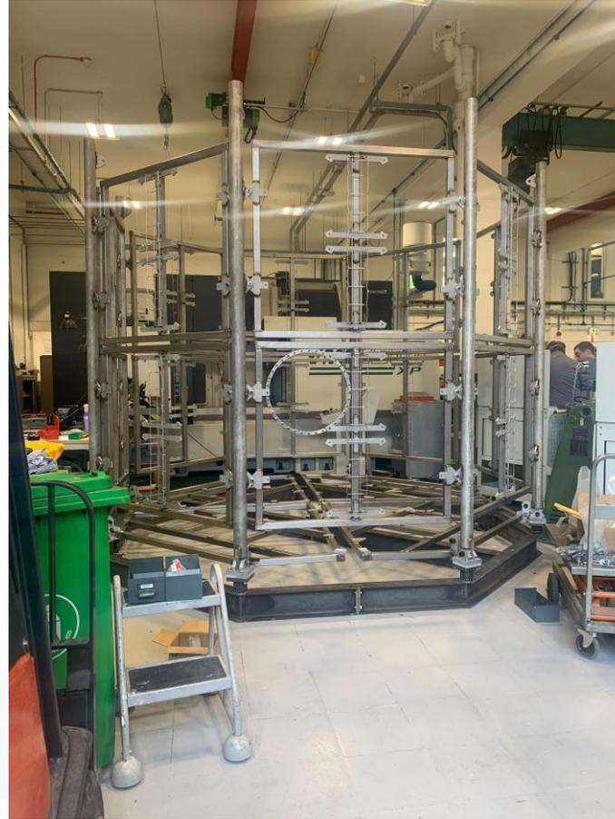
Production of the 316L PSUP was undertaken by Liverpool University workshop. This is modular for the later inclusion of advanced photosensors.
