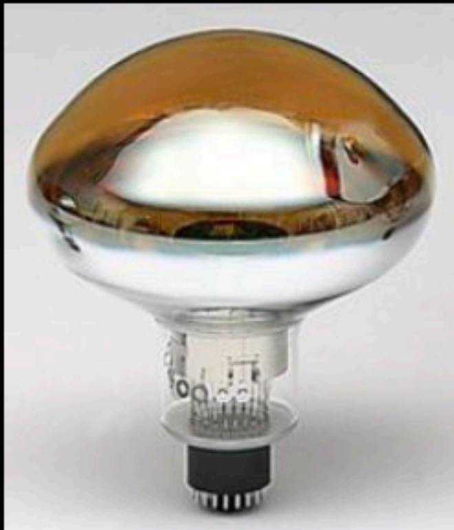
10-inch PMT R7081 IceCube Collaboration, NIM A 618 (2010)
