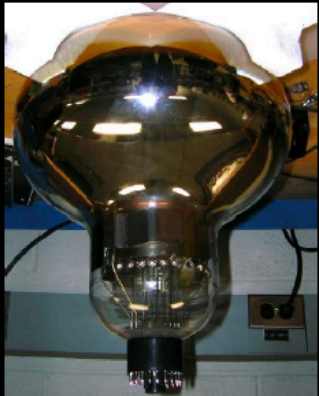
12-inch PMT R11780 J. Brack et al., NIM A 712 (2013)
