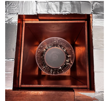
0.9 kg of high-purity Nb loaded on the Ge detector at SURF
