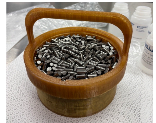
3.6 kg of high-purity Nb deployed at PNNL
