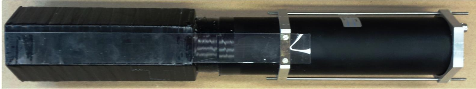
silicone oil coupling, quartz window, PMT
