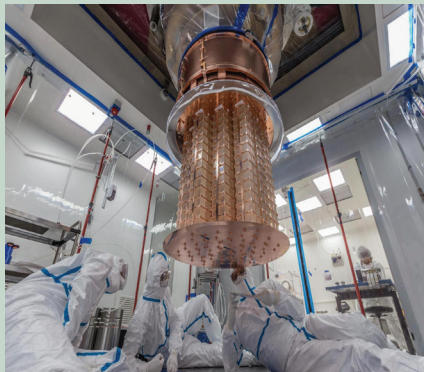
Figure 4: The CUORE experiment used radon-free environments to assemble and install the bolometer towers. | Image reproduced with permission from Yury Suvorov, University of California Los Angeles and Gran Sasso National Laboratory (Italy), and the CUORE Collaboration.
