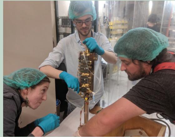
Figure 1: ADMX personnel assemble a cryo-electronics package containing a JPA and a TWPA for their axion search. | Image reproduced with permission from Gray Rybka, University of Washington.
