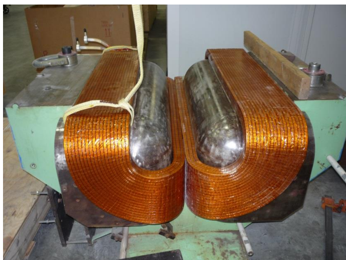
100T coil with CTD-101K (photo courtesy of Everson Tesla)
