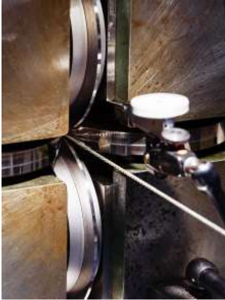
~150 m 6-strand cable (strand d = 0.7 mm) fabricated@LBNL
