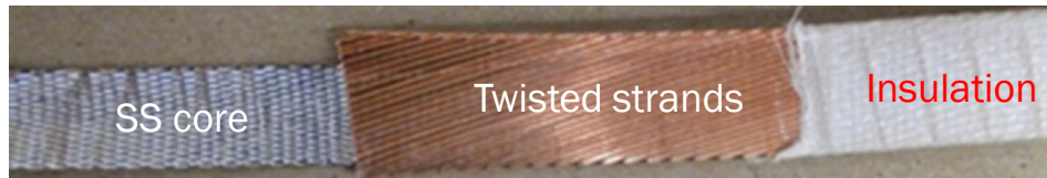
1 mm RRP150/169 28-strand cable with SS core
