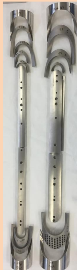
Ti poles and spacers, SS saddles
