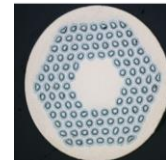
0.7 mm RRP108/127 40-strand cable with SS core
