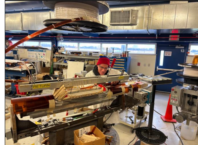
Coil#2 winding in progress
