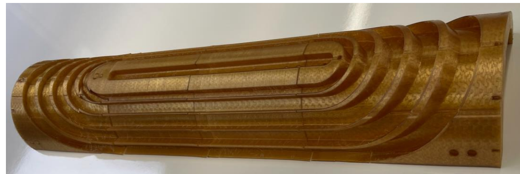
SMCT layer 2 printed from ULTEM
