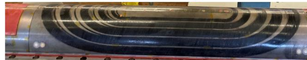
Coil view after epoxy impregnation
