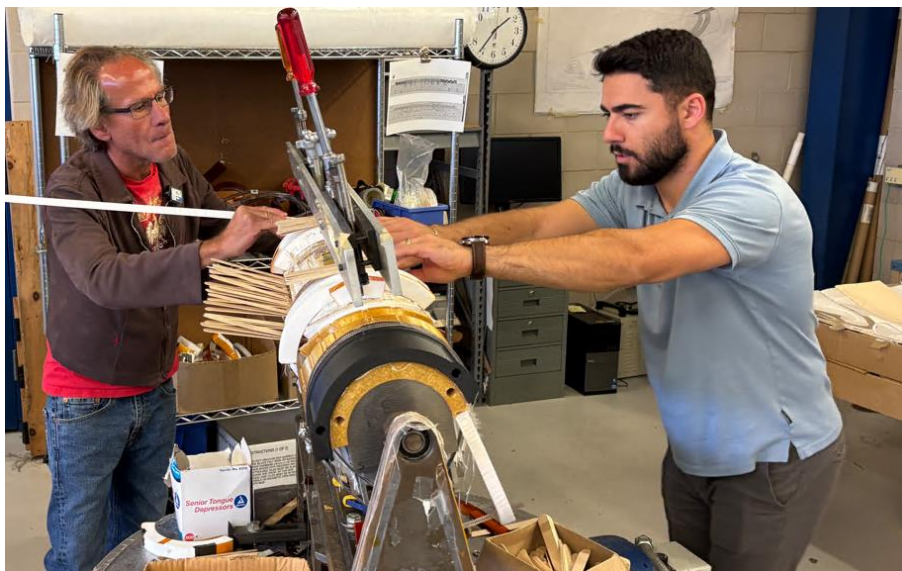
New winding setup for the flex mandrel and rigid cable
