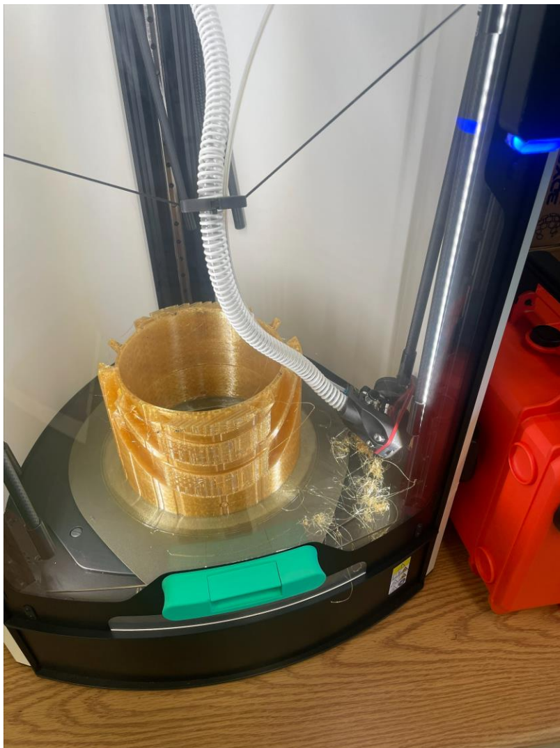
Printing of mandrel from ULTEM
