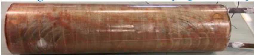
Impregnated coil a foot long
