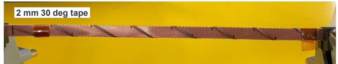
Figure: Sample fabrication of 2mm tapes at 45 deg and 30 deg lay angles
