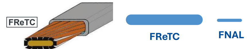
Figure: FReTC cable, developed by M. Takayasu, geometry compared to new proposed cable (schematic provided by C. Navarro)
