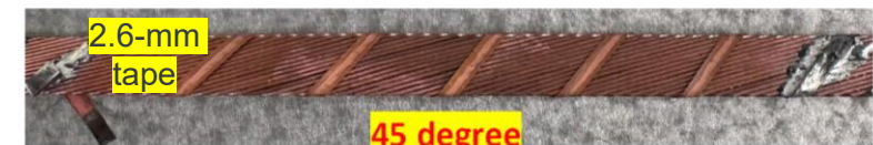
Figure: FReTC cable, developed by M. Takayasu, geometry compared to new proposed cable (schematic provided by C. Navarro)
