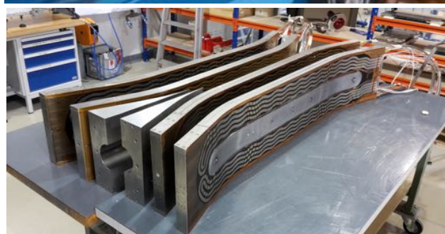
2018: FRESCA2 (CERN/CEA) at CERN 14.6T at 1.9 K, 100 mm
