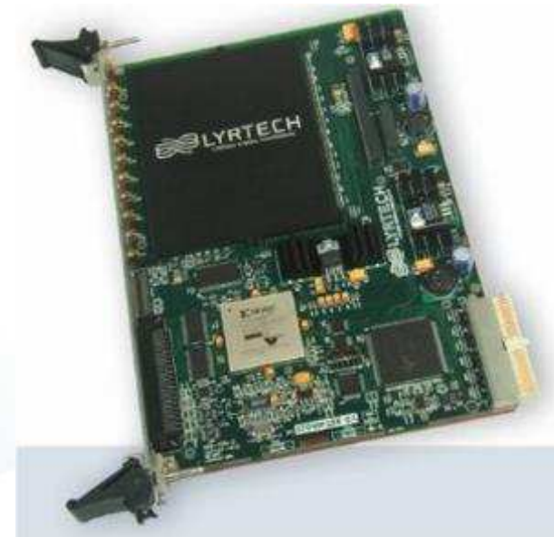
Digital board: VHS-ADC from Lyrtech
