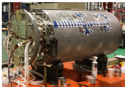
MDPCT1 cos-theta dipole design and technology demonstrator
