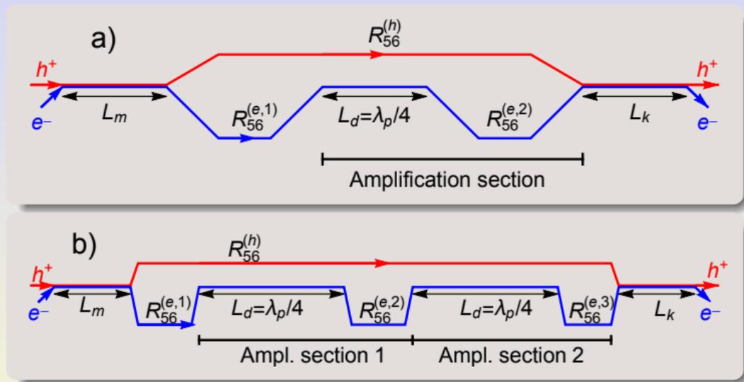
The main advantage of MBEC is its broadband amplification as compared to the narrow-band FEL CeC. The effective bandwidth of this amplifier is tens of THz.
