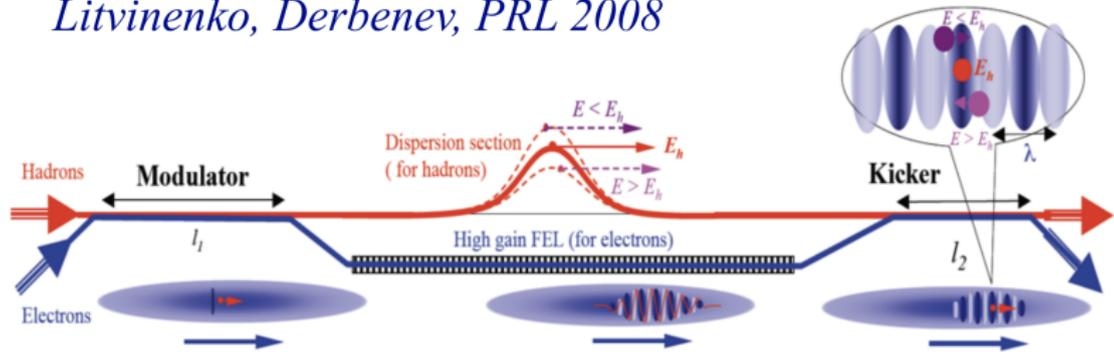
A proof-of-principle experiment was conducted at BNL, however, the cooling was not observed (because of the large noise in the electron beam).
