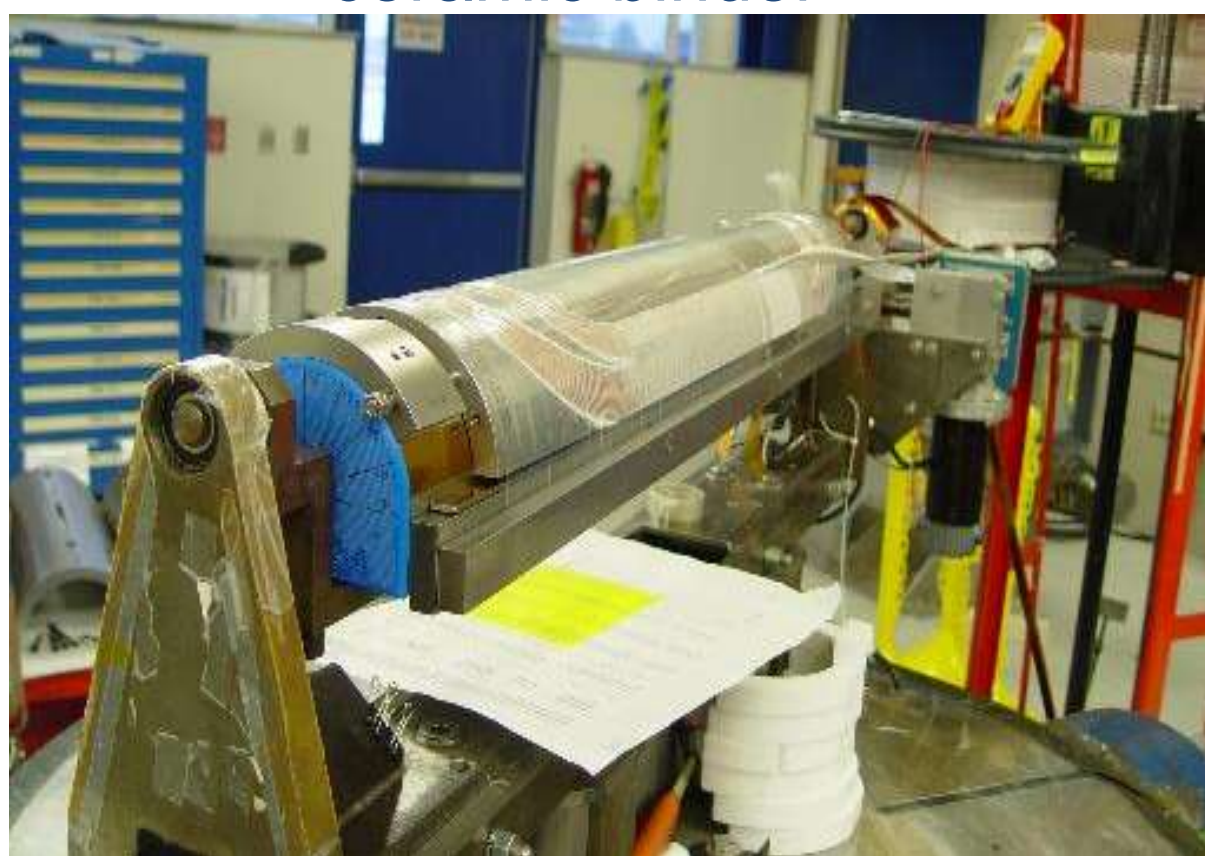
Coil winding and curing using ceramic binder
