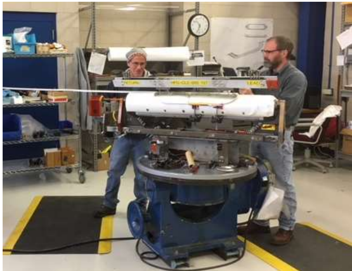
Coil winding and curing using ceramic binder
