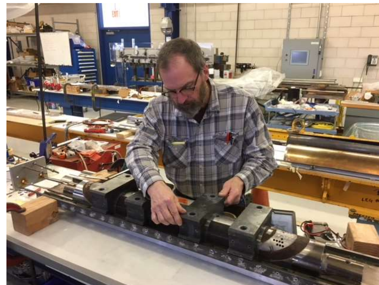
Coil lead splicing, epoxy impregnation
