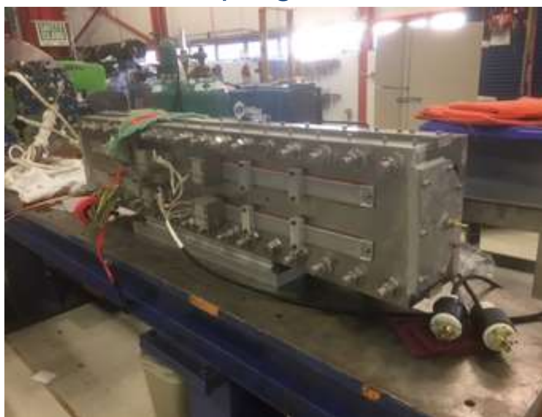
Coil lead splicing, epoxy impregnation
